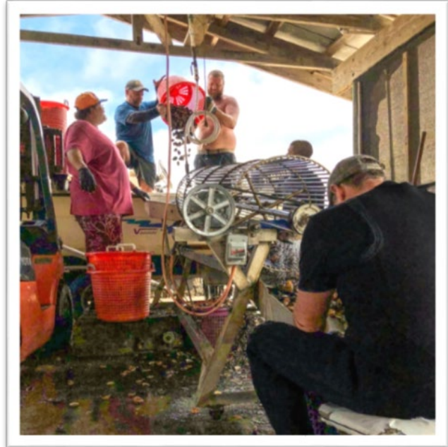
Figure 1. After a long day of planting, hauling and harvesting - clam producers tumble and wash product prior to sorting, bagging and distributing. This crew reduces back strain by trailering their boat to an elevated position relative to the tumbler to off-load 100-pound baskets of product into the hopper (avoiding having to lift from ground level). Heavy lifting is also done with the assistance of a second person, when possible.
