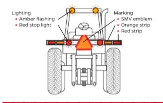
agricultural vehicle owners to create a pattern of lighting and marking that is recognizable at a distance. This additional information for other drivers is very important. It signals to them at a greater distance that a large, unusually shaped vehicle is ahead of them on the road, and they need to slow down and take proper precautions.
